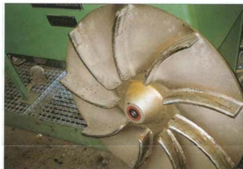
Fig. 5: Fan impeller showing wear after 1 week of operating time
